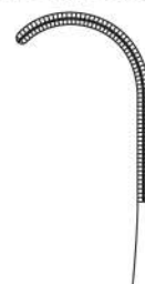
ST22-279-08 16.5 cm jaw length 3.5 cm depth 1.3 cm Fig. 8
