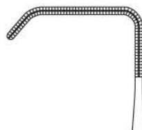
ST22-279-07 16.5 cm jaw length 3.2 cm depth 6.8mm angled 90° Fig. 7
