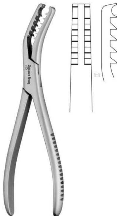
Semb Bone Holding Forceps ST15-681-19 19 cm without ratchet curved sideways deep teeth
