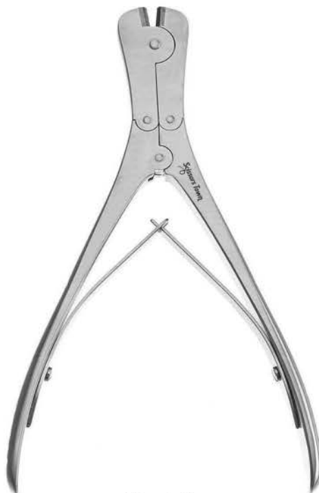
Wire Cutter ST15-899-17 17cm carbide inserts, double action. Max capacity. 1.6mm 062"
