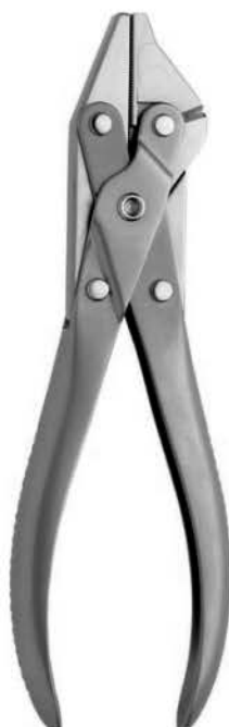
Flat Nose Plier ST15-602-18 18.5cm parallel grip, incorporated cutter, for hard wires up to 1.6mm
